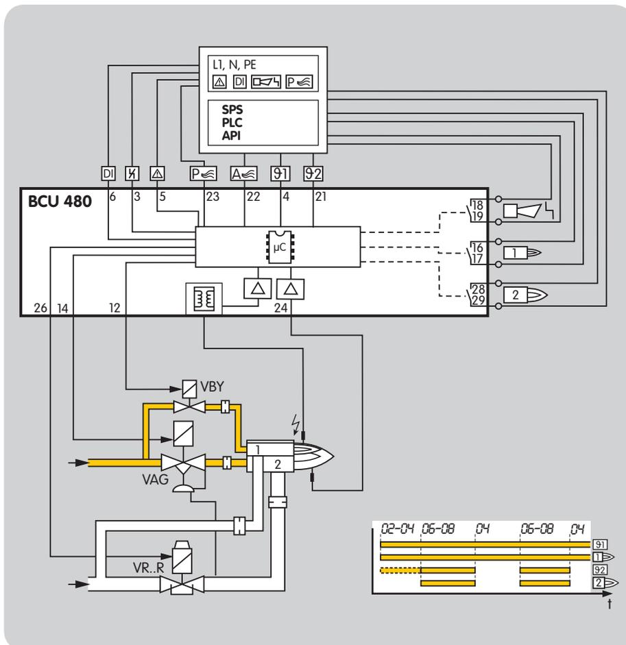
Stage-controlled main burner with permanent pilot burner
