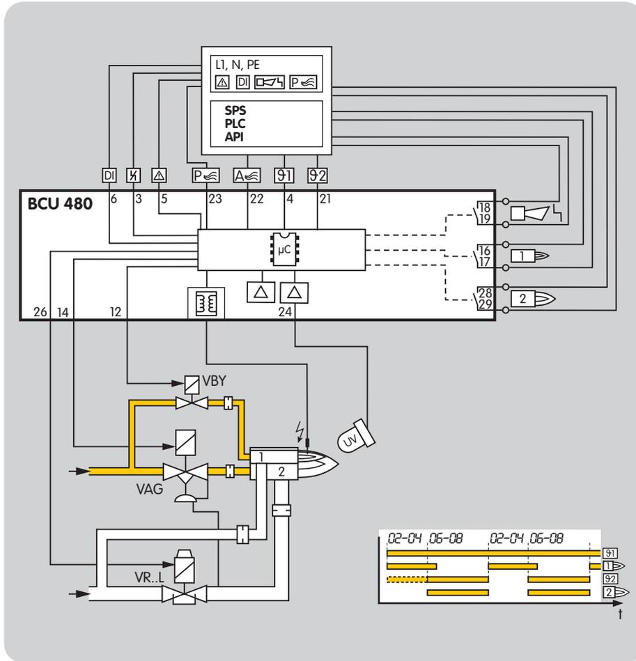
Stage-controlled main burner with alternating pilot burner
